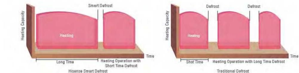
The Hisense Smart Defrost process is only performed when needed which reduces energy waste by eliminating the unneeded defrosting process. Enjoy maximum comfort in heating operation by reducing defrosting time.
