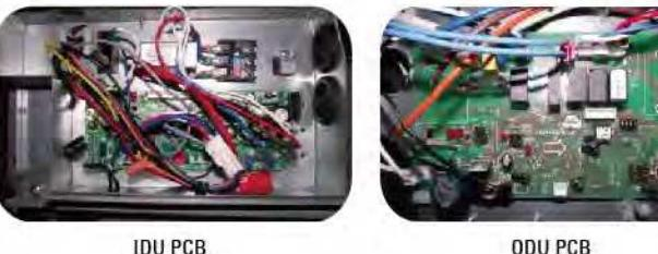
More concisely control: By Dual PCB control, the system reads the operating status timely in order to achieve optimal control, smart defrosting etc.
